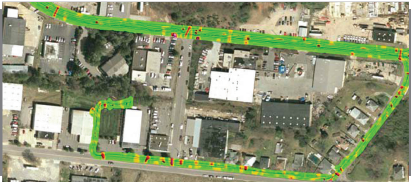
Example data obtained along streets in Raleigh, NC, superimposed upon an aerial photograph of the area. The survey was undertaken to detect all utility lines (water, sewer, powerline, telephone and fiber optic cables) buried under the road. Faint black lines indicate the ground track of the array.
