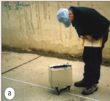
Figure 11. (a) Gravity survey in a palace compound. (b) A gravity anomaly under flooring led us to a palace wine cellar.
