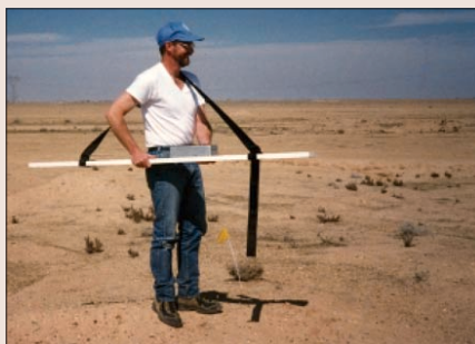
Figure 3. A handheld electromagnetic sensor was one of the workhorse geophysical instruments to cover large areas very quickly.
