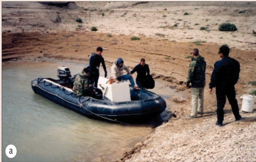
Figure 10. (a) The Navy's Zodiac inflatable boat was frequently used for conducting geophysical surveys over water. Typical sensors included a side-scan sonar, magnetometers, and, at times, electromagnetic sensors. (b) Anchored buoys were used to mark anomalies over water in real time. A recovery team dove into the murky river to inspect each anomaly and retrieve the finds.
