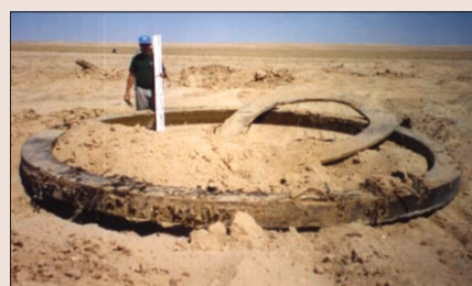
Figure 4. A large copper tube assembly made for isotope separation for the Iraqi nuclear program. A magnetometer once missed it because of its nonferrousness. The electromagnetic data led to its excavation.
