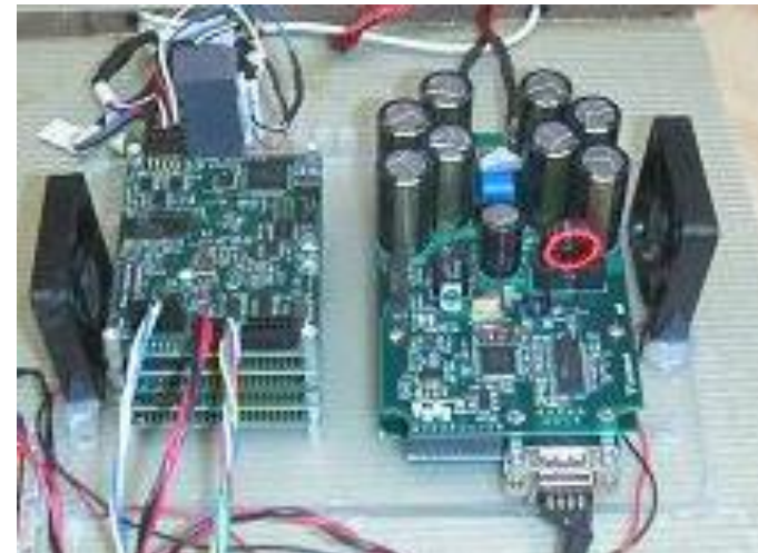
Geophex's multi-channel transmitter and receiver electronics
