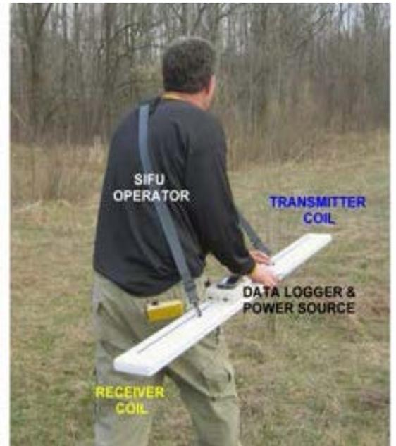
GEM-2 Electromagnetic Induction Survey in Progress
