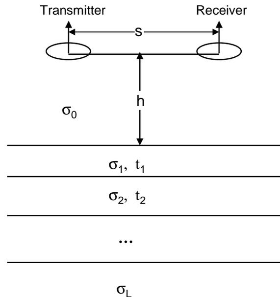
FIG. 1. Geometry of the EM sensor over a layered earth, where  $\sigma$  is the conductivity,  $t$  is the thickness of each layer, the subscripts stand for number of layers,  $s$  is the coil separation, and  $h$  is the sensor height.
