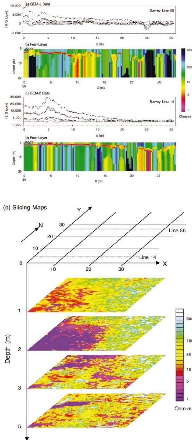
FIG. 10. Two GEM-2 profiles, (a) and (c), from a survey in Hutchinson, Kansas. The solid curves stand for in phase, and the dashed lines are the quadrature at 18270, 7290, and 2430 Hz. The depth sections (b) and (d) are based on 1D inversion using a four-layer model. Resistivity slice maps (e) at depths of 1, 2, 3, and 5 m.
